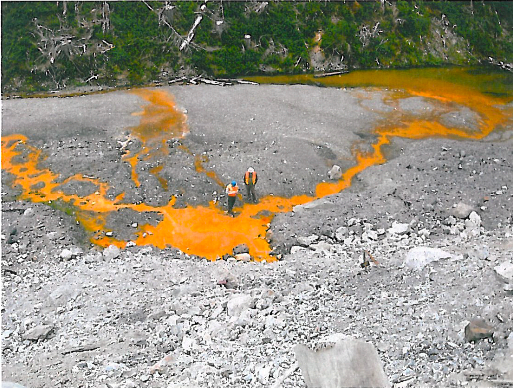
Kensington Figure 2. Acidic waste rock seeps flowing into the tailings facility, 2013. See Table 1 for water quality results. Source: ADEC, 2013. Notice of Violation. Kensington.NOV.ADEC 2013.pdf [6]
