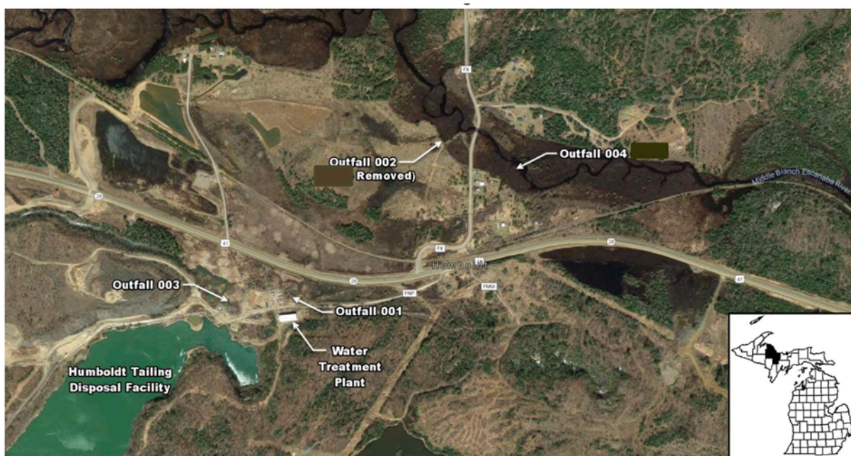
Eagle Figure 2. Humboldt Tailings Disposal Facility (HTDF) treated effluent discharge locations: Outfall 001 and Outfall 003 (wetland contiguous to the Middle Branch Escanaba River) and Outfall 004 (direct discharge to the Middle Branch Escanaba River). Source: Michigan Dept. of Environment, Great Lakes, and Energy, 2022. Fact Sheet, Permit No. MI0058649. Eagle.NPDES Fact Sheet.EGLE 2022.pdf [4]
