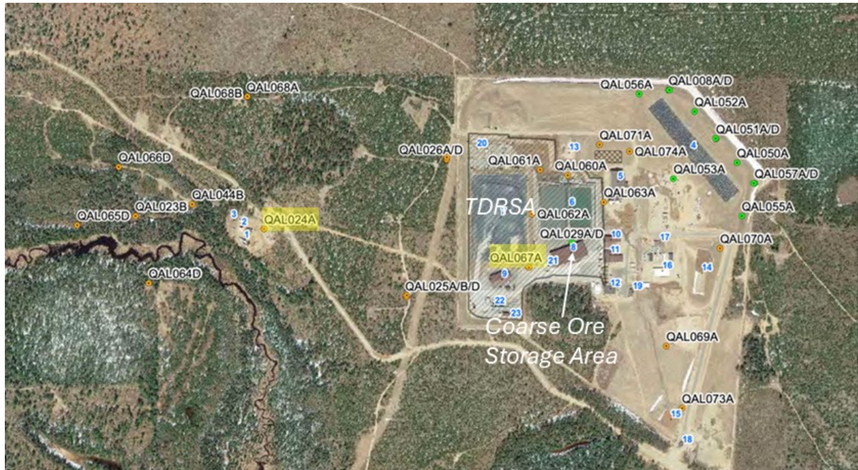
Eagle Figure 4. Mine site groundwater monitoring well locations. Discharge permit wells are shown in green, and mining permit wells are shown in orange; the treated water infiltration system is #4 on the map. Water quality results are plotted for the two compliance wells highlighted in light yellow.
