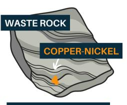
Waste rock full of sulfates exposed to air and water, becomes sulphuric acid.
