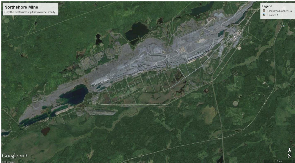
Figure 18: Google Earth image of the Northshore Mine. The westernmost pit has water while pits to the east are dewatered.
