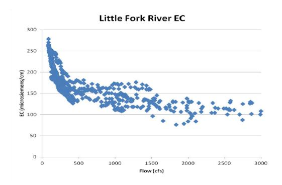
Figure 17: Relation of electrical conductivity with flow at the Little Fork River at Littlefork MN gage (#05131500). Years 1980 through 1983. Data source:
